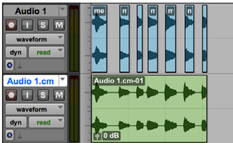
Source Track (top) and Committed track (bottom) with Commit set to Selected Tracks and the Consolidate Clips option enabled
